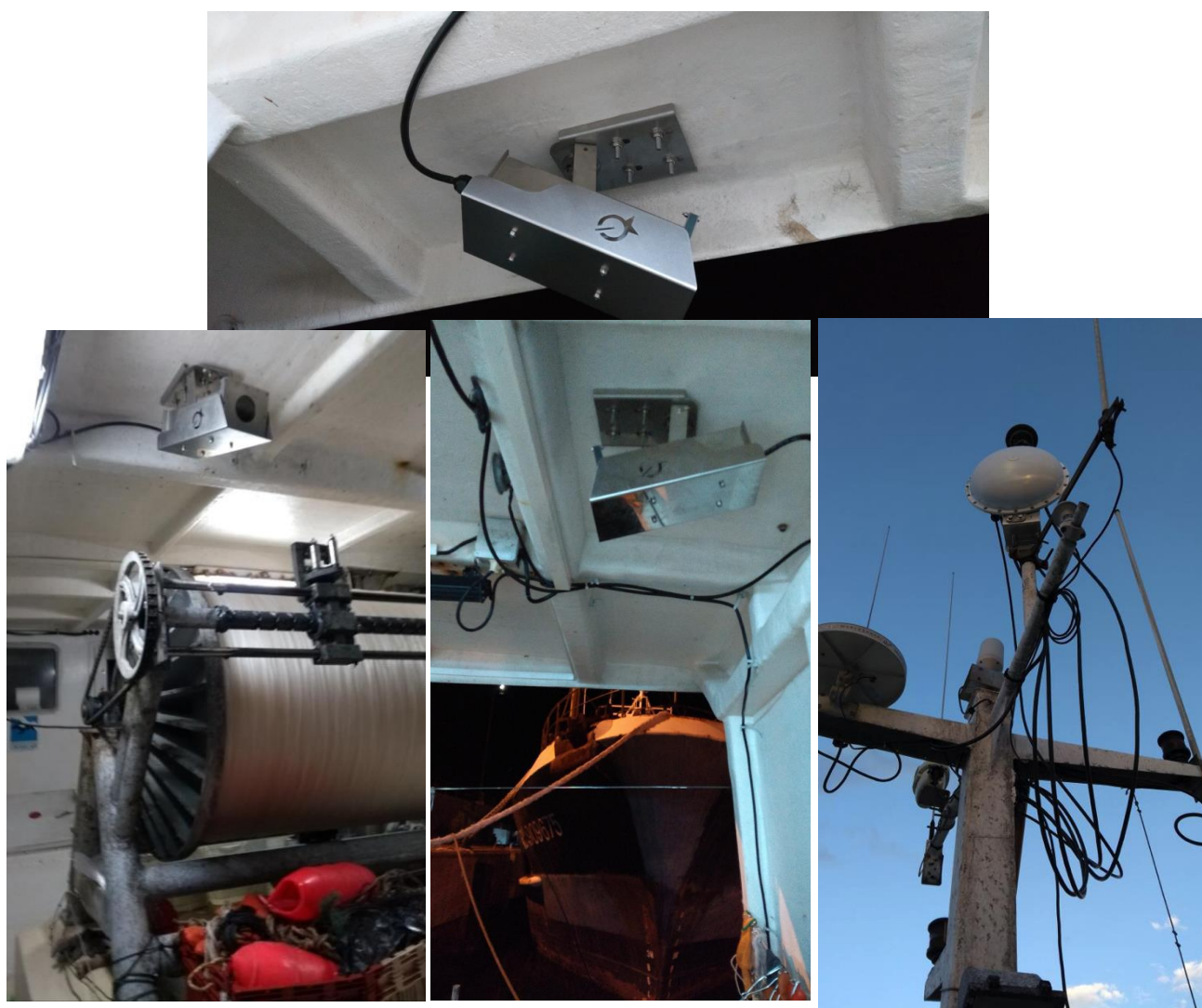
Figure 3 – Cameras (1 top, 2 below left, 3 below middle – number refers to table 3) and main unit at the mast installed on “Le Grand Morne”.
