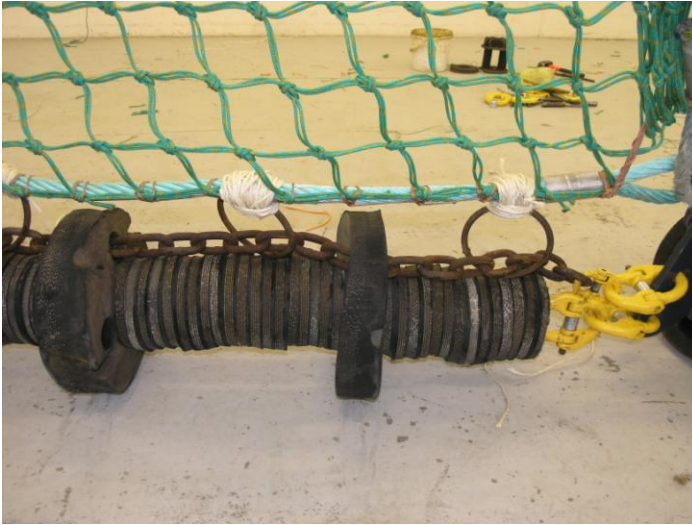
Figure 1. GOV lower wingend showing 5mm double PE guard netting and Ground gear D hoppers
