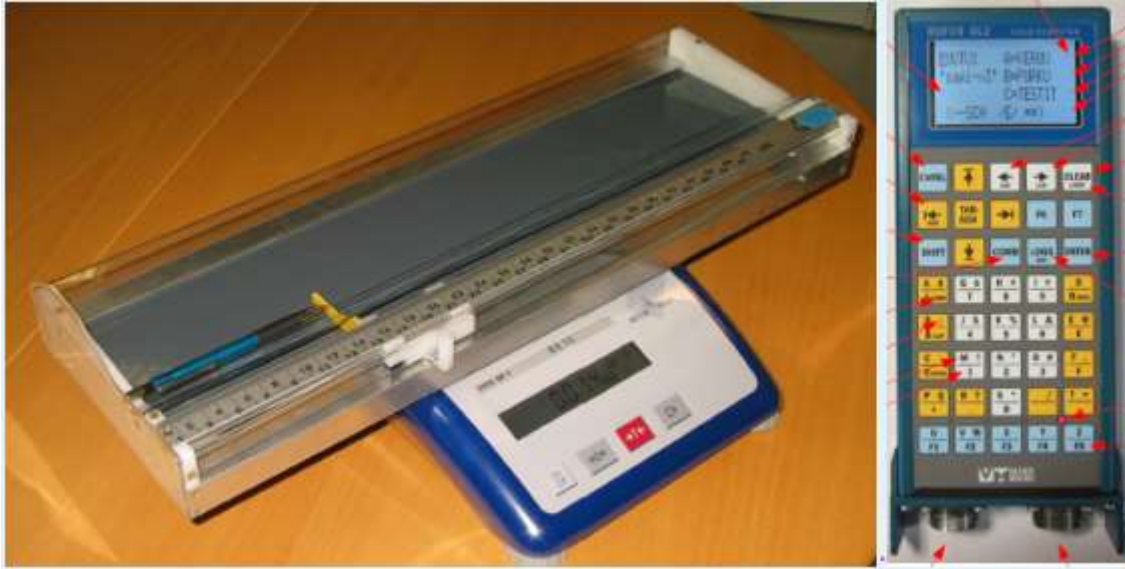
Figure caption: On the left: The measuring and weighing units. On the right: The Data logger.
