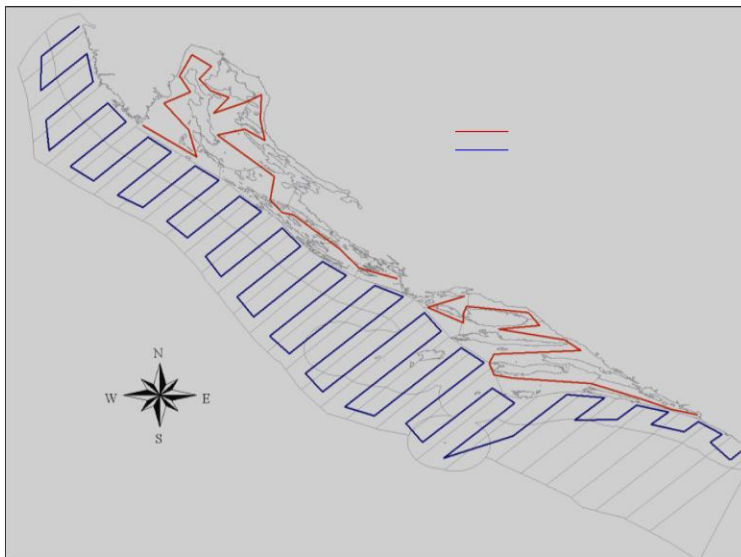
Figure 2. Acoustic Survey Design in the Eastern Adriatic Sea (Croatian waters). – i.e. Eastern part of GSA 17: 30 parallel transects in the open sea area in 43°-223°direction up to mid-line, and randomly positioned transects in channel area (inner sea).
