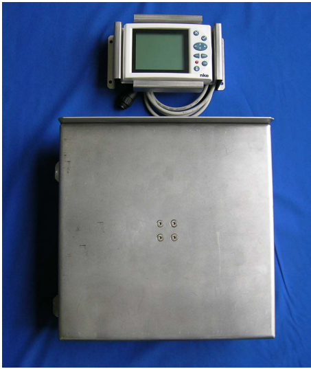
Figure 7.3 Recopesca weigh-scale (pan and command module)
