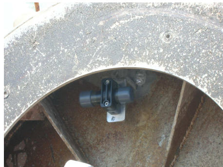
Figure 7.2 The hauler revolution counter fixed in a gill-net hauler
